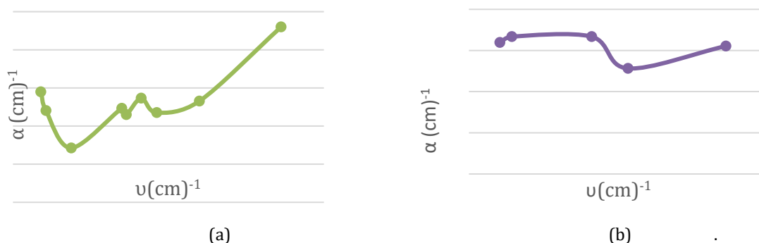
Figure (5): represents changes of absorption coefficient as a function of vibrational frequency SnO 2 (b) ZnO (a).
